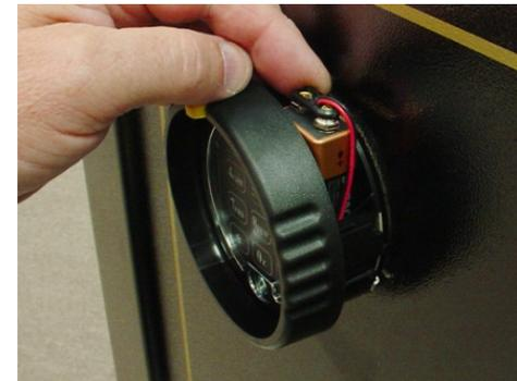
Install a 9 volt alkaline battery, Duracell is recommended. To install the battery, pull the lock/unlock indicator tab out slightly and turn the ring counterclockwise (left) to reveal the battery storage area and battery connector. Attach the battery then push the ring back toward the base while turning clockwise (right). The ring will 'click' when properly seated.
